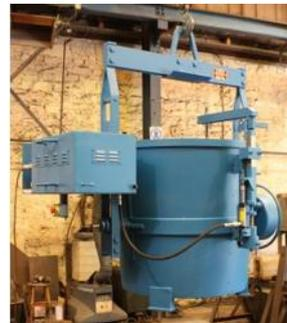
ZH Bottom-Pouring Ladles, complete with Remotely Operated Hydraulic Ropastop Bottom Pour Slide System.
