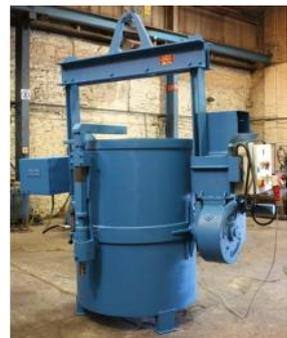
ZH Bottom-Pouring Ladles, complete with Remotely Operated Hydraulic Ropastop Bottom-Pour Slide System and Motorised Remotely Operated Roperlok Gearbox.
