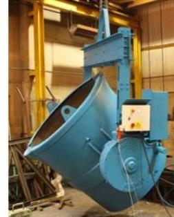
ZH Lip-Pouring Ladles, complete with Motorised Remotely Operated Roperlok Gearbox.
